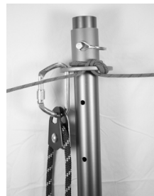
fig. 25: Lash Ring atop gin pole as main attachment
