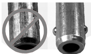
fig. 31: Left pin - retired due to wear and detent pins not properly working; Right pin - in good working condition
