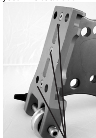
fig. 22: Do not remove these screws
