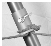
fig. 24: Lash Ring used near foot section for increased stability
