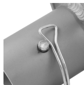
fig. 3: Improperly secured Leg Coupling Pin
